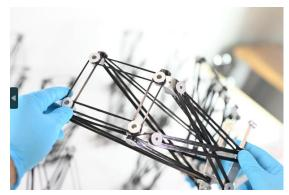
GRAM is based on AI-driven topology optimization for 3D design and simulation, combined with a six-axis robotic system that handles material placement and resin application. The process creates a 3D structure where bush components are linked by fiber materials, with the bushes serving as end points. The structure is solidified with resin, resulting in a lightweight yet robust component. A wide range of fibers can be used, including carbon fibers, natural flax, basalt fibers, rayon, and glass.
